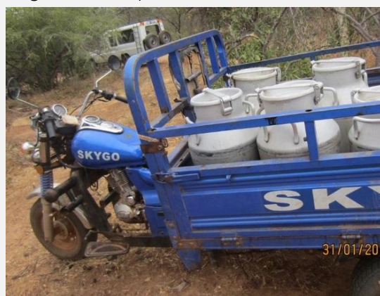
Figure 16: A modified motorbike dedicated to transporting milk to collection centre.
