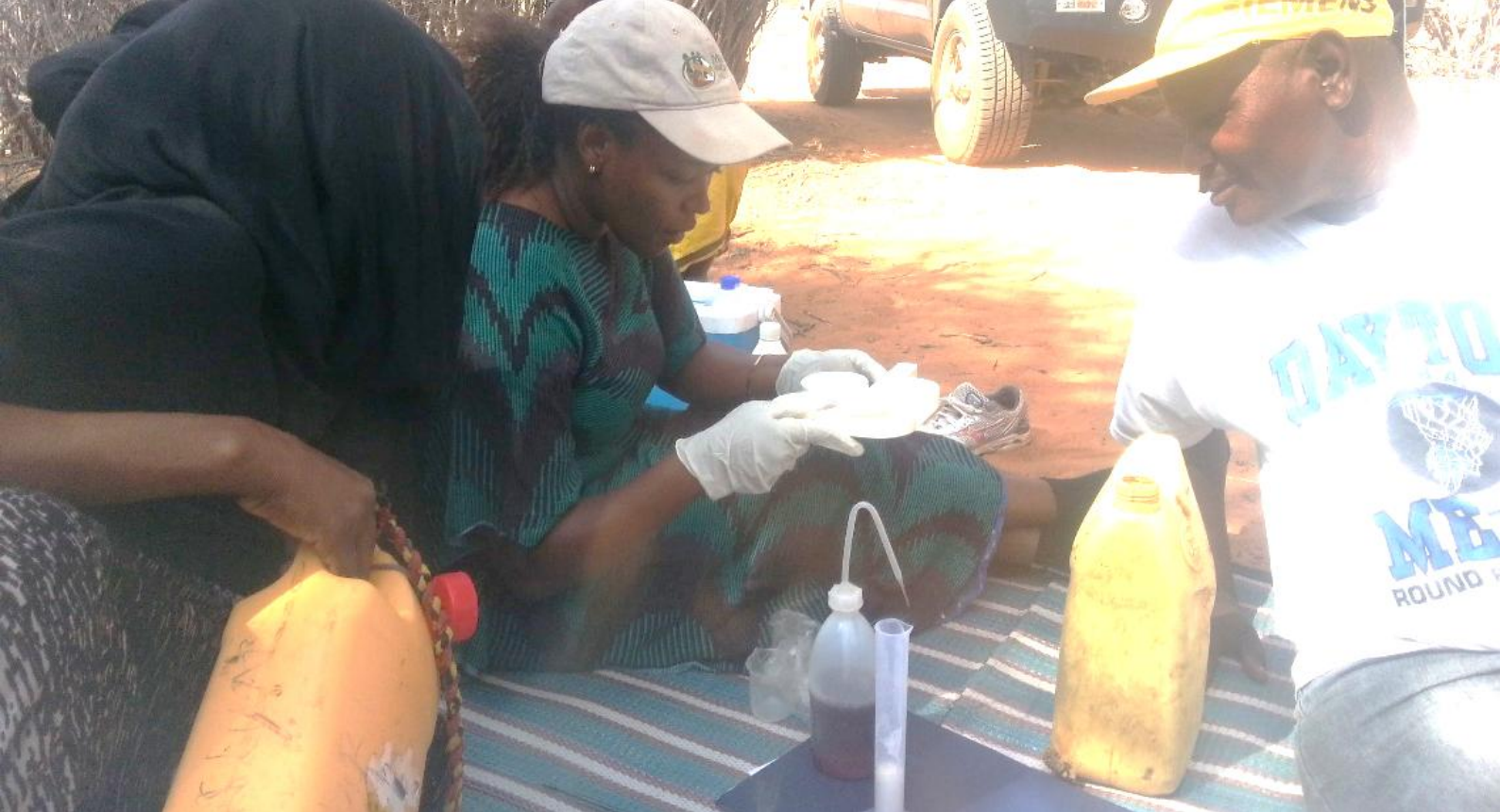
Figure 6: Camel milk quality testing using CMT reagent and paddle at primary trader level
